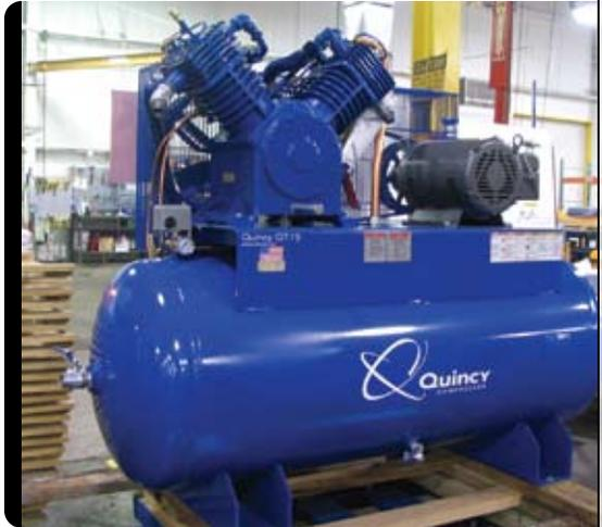
*Quincy Compressor is a leading manufacturer of industrial compressor systems for industrial and commercial applications. The cylinder head on this unit, which is ready to ship, was honed on an HMC.*
