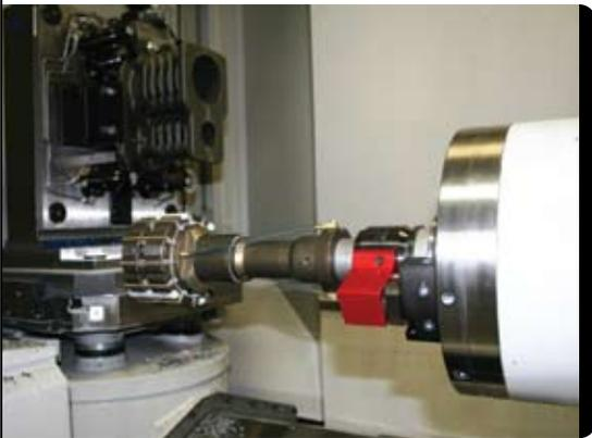
Unlike most dedicated honing machines, the honing tool operates horizontally in the spindle of the HMC. The red attachment at the base of the honing tool's shaft is the coupling for the air line that is used to gage bore size during the honing process.
