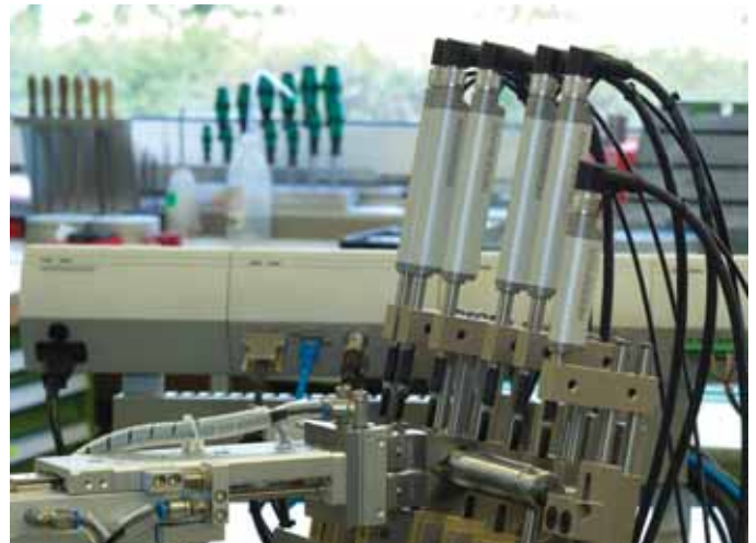
Fig. 2. A typical application: Measuring the diameter and length of a shaft automatically.
